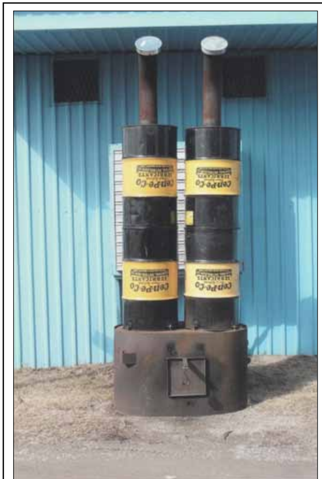
Grawmondbeck's Competition Engines in Mason City Iowa used Cen-Pe-Co oil barrels, provided by Cen-Pe-Co's Mark Bosma, to fabricate a muffler for their engine dyno. There is more than one way Cen-Pe-Co helps engines make more power.
